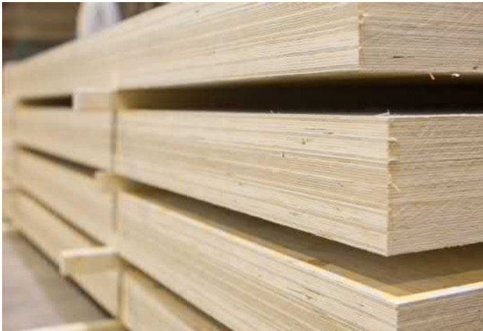
Figure 3.4. Storage of LVL packages
