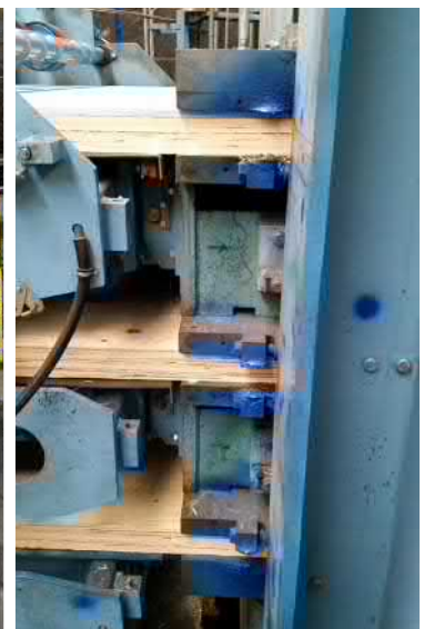
Figure 1.43. Feeding LVL billets into 3-level hot press.
